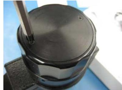
2. The silver Philips screw in the center of the knob (inside red circle at right) should NOT be loosened. If it is loose at all, snug it up as much as possible. This screw is not relevant for tension adjustment, and must remain tight to avoid knob play.
