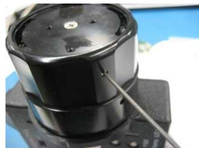
4. The piece with holes that is accessible through the grooves in the shell is the pressure washer housing. With the set-screws loose, it should spin with respect to the outer knob shell. Hold the knob shell stationary with your hand:
