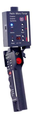
The Radio Micro Force module works in conjunction with either Analog V+F or Digital Micro Force models and the 3- channel FI+Z system to provide wireless zoom operation. When the Radio Micro Force module is powered, the FI+Z wireless network recognizes its presence and hands over to it control of the zoom function. When the unit is powered down, zoom control reverts back to the FI+Z HU3 Hand Unit.
