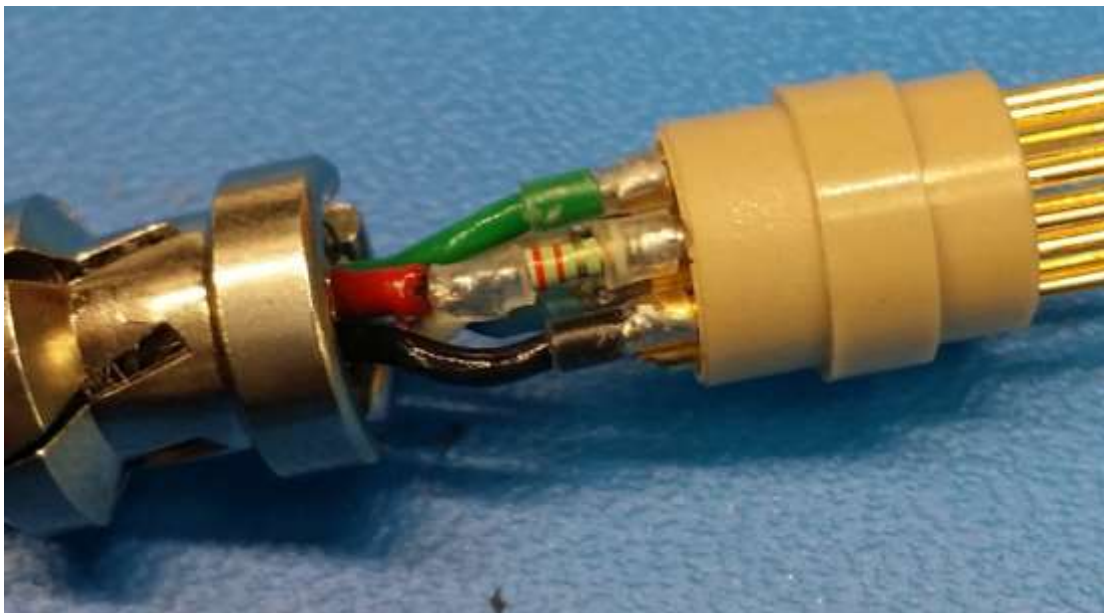
Figure 1 - 2Ω series resistor installed on +12V line
