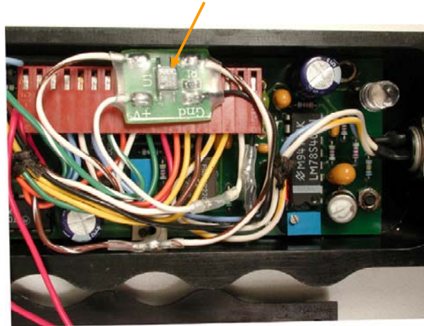
Opto-Isolator circuit board
